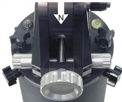
Mount centered in azimuth.
