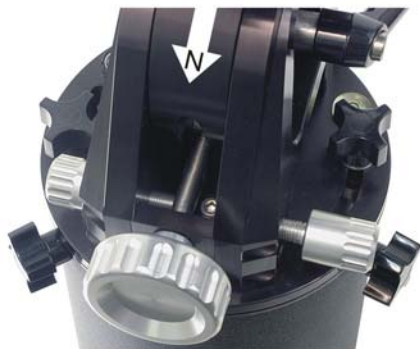
Azimuth adjusted to the east.
