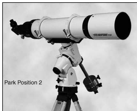
Park Position 2 Scope is level and pointing east, RA axis vertical, Dec = 0
