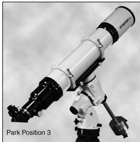
Park Position 3 Scope is pointing to the pole. RA axis vertical, Dec = 90
