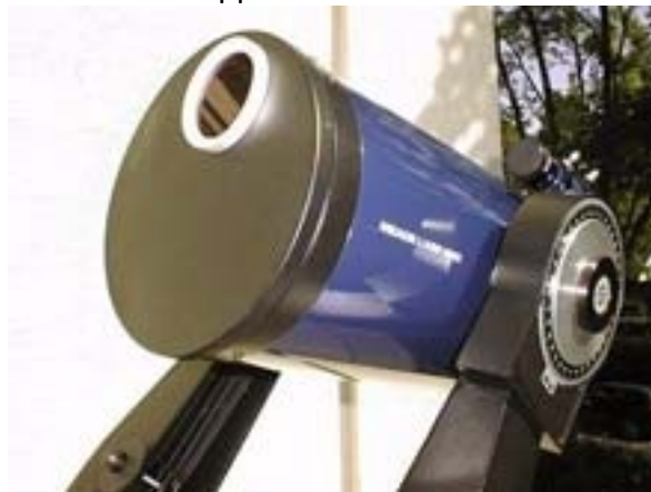
Figure 14: Off-axis Energy rejection filter.
