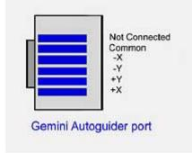
**IMPORTANT:** There are two different versions of the Gemini Autoguider port hardware. The versions can be distinguished by the type of connectors used for the motor cables. The older Gemini version uses RJ-45 modular connectors, and the newer version uses 6-pin DIN connectors. The primary difference between the versions is that the older version does not directly support autoguiders with TTL output, but the newer version does.
