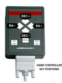
**Menu Mode:** Press the MENU button and "MENU" is displayed. The DEC+/– buttons scroll through the possible selections, the RA+ button selects items (like a computer's 'enter' key), and the RA– button usually goes back to the previous selection (like a computer's 'back arrow'). Pressing the MENU button again returns Gemini to Telescope Control Mode for guiding, centering, and slewing the telescope.
