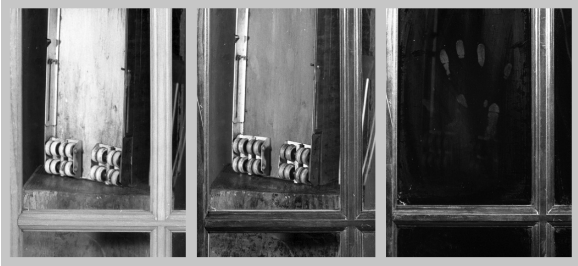
Figure 8. Latent handprint on glass window. Left – visible monochrome image. Middle – 350nm, Right – 310nm image.
