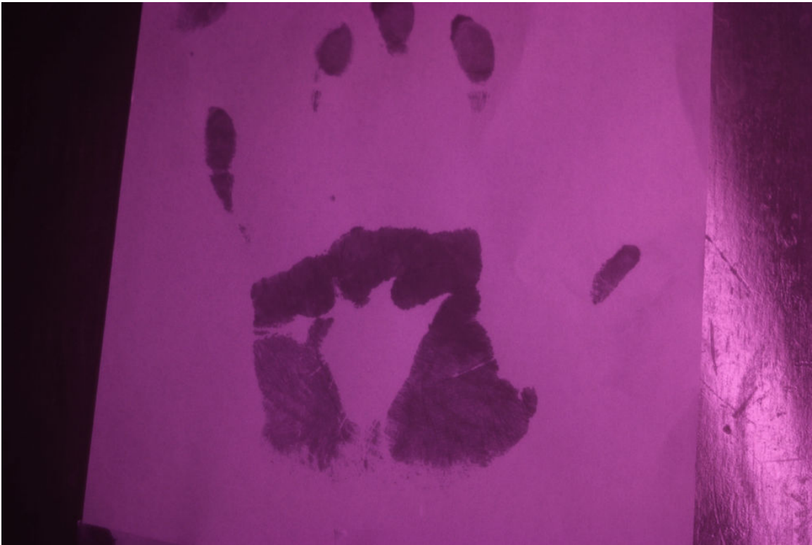
Figure 26. RGB composite image of handprint on paper. Illumination is 365nm.
