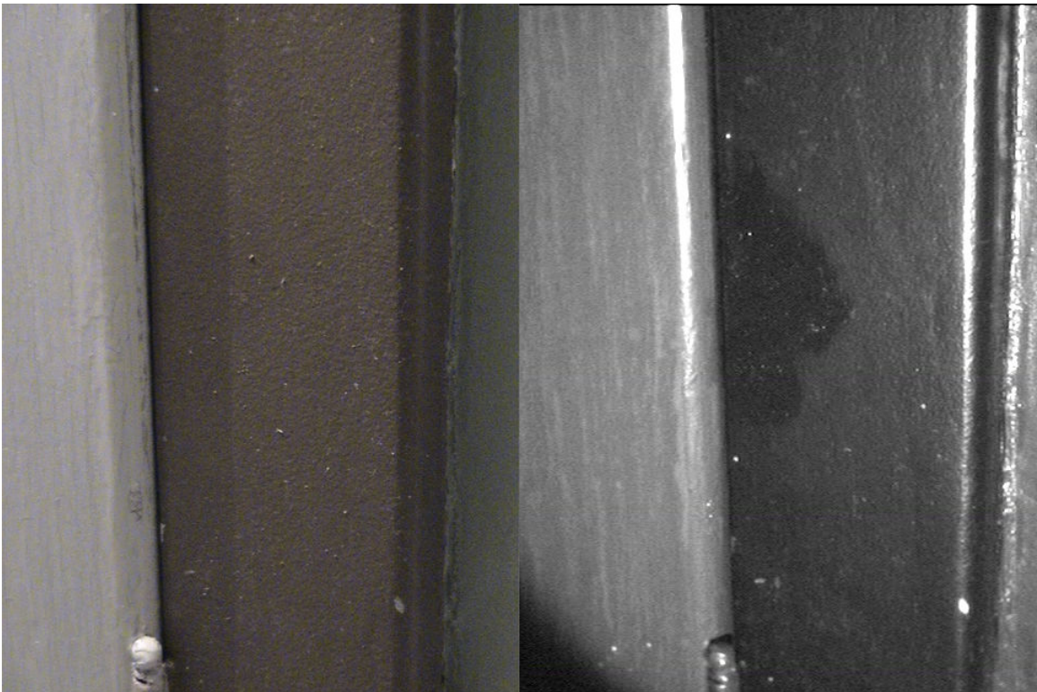
Figure 15. Unknown oil stain on brown painted metal. Left – color, right – near-UV
