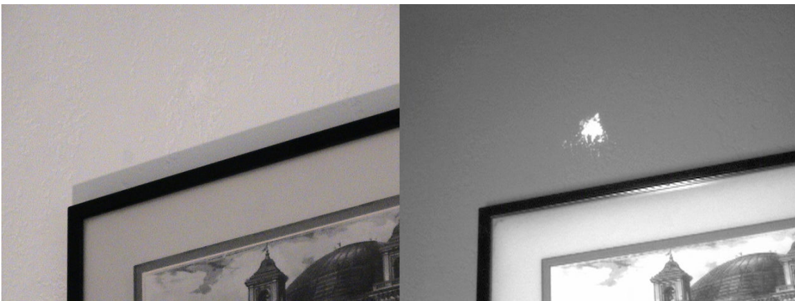
Figure 13. Spackle on walls painted with white latex paint. Left – color, right – near-UV
