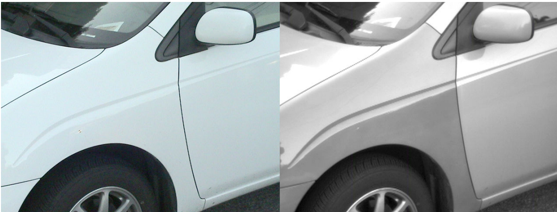
Figure 10. A repainted front driver's side fender on a Toyota Prius. Left – color, right – near-UV
