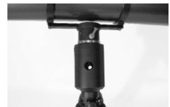
**Figure 7.** The optical tube must be at a 90° angle to the R.A. axis in order to view through the polar axis finder.
