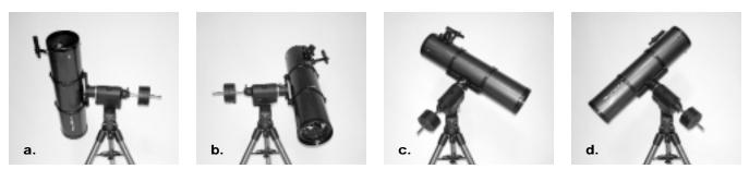
**Figure 10a-d.** These illustrations show the telescope pointed in the four cardinal directions. (a) north, (b) south, (c) east, (d) west. Note that the tripod and mount have not been moved; only the telescope has been moved on the its R.A. and Dec. axes.
