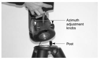
**Figure 2.** Orient the equatorial head so that the post on the tripod lines up with the azimuth adjustment knobs on the equatorial mount.
