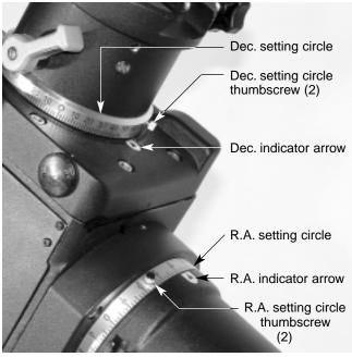
Figure 9. The R.A. and Dec. setting circles.
