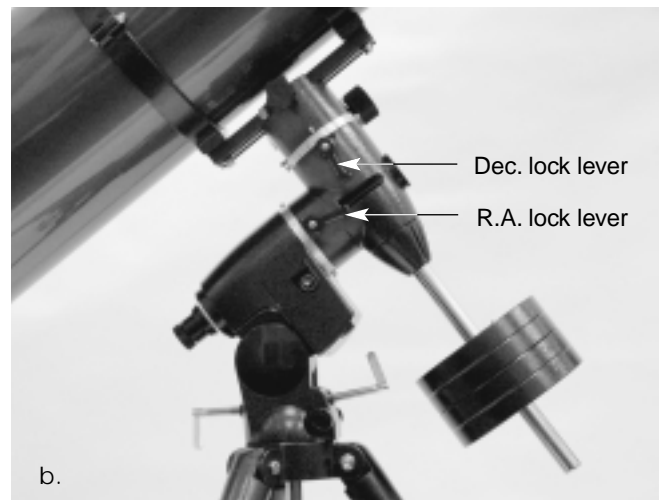
Figure 4. The SkyView Pro Equatorial Mount, shown from both sides.
