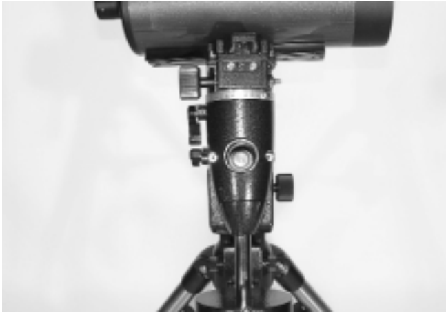
Figure 10. The optical tube must be at a 90° angle to the right ascension axis in order to view through the polar axis finder.
