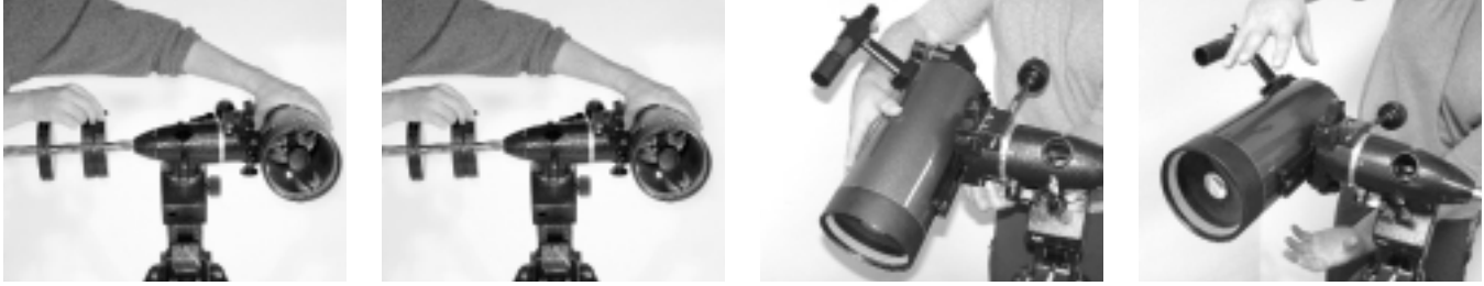
Figure 4a-d. Proper operation of the equatorial mount requires that the telescope tube be balanced on both the Right ascension and Declination axes. (a) With the R.A. lock lever released, slide the counterweights along the counterweight shaft until it just counterbalances the tube. (b) When you let go with both hands, the tube should not drift up or down. (c) With the Dec. lock knob released, loosen the tube ring lock clamps a few turns and slide the telescope forward or back in the tube rings. (d) When the tube is balanced about the Dec. axis, it will not move when you let go.
