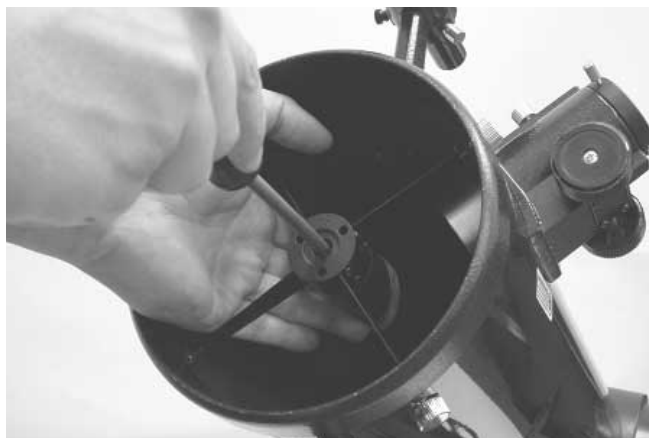
Figure 15. To center the secondary mirror under the focuser, hold the secondary mirror holder in place with one hand while adjusting the center bolt with a Phillips screwdriver. Do not touch the mirror's surface!
