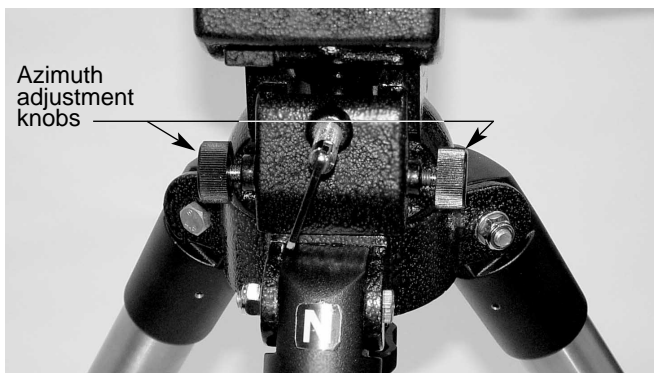
Figure 9. For polar alignment, position the tripod so that the "N" label at the base of the mount faces north. The azimuth fine adjustment knobs above it are used to make small adjustments to the mount's azimuth position. Be certain to loosen the tripod attachment knob on the central support shaft before adjusting these knobs.
