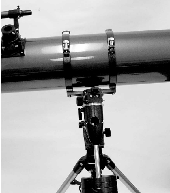
Figure 11. The optical tube must be at a 90° angle to the right ascension axis in order to view through the polar axis finder
