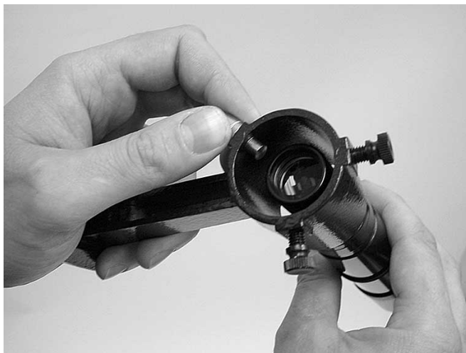
Figure 3b. Pull back on the tensioner and slide the finder scope into its bracket until the O-ring is seated in the bracket ring.
