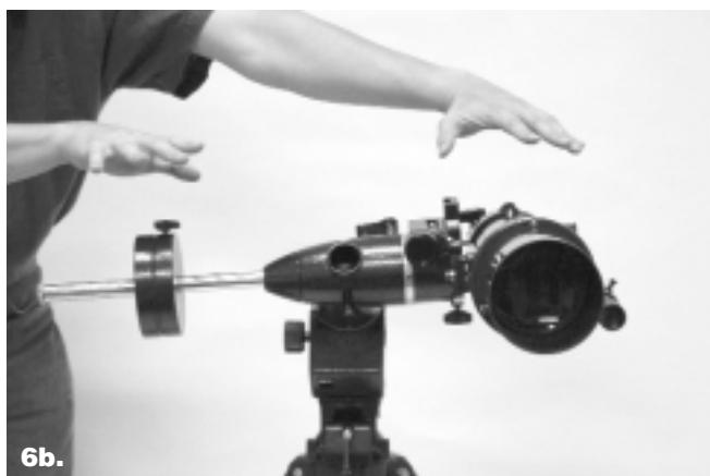
Figure 6a, 6b. Proper operation of the equatorial mount requires that the telescope tube be balanced on the R.A. axis. (a) With the R.A. lock lever released, slide the counterweights along the counterweight shaft until it just counterbalances the tube. (b) When you let go with both hands, the tube should not drift up or down. The telescope tube should already be balanced in the Dec. axis if you have properly centered the 1/4" mounting block between the tube rings.
