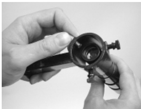
Figure 3b. Pull back on the tensioner and slide the finder scope into its bracket until the O-ring is seated in the bracket ring.
