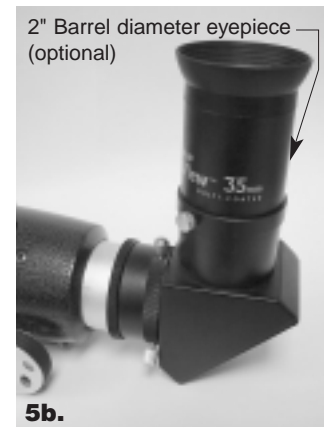
Figure 5a. and 5b. To use 1.25" barrel diameter eyepieces, the 1.25" adapter must be installed in the 2" star diagonal. 5b. To use 2" eyepieces, remove the 1.25" adapter.
