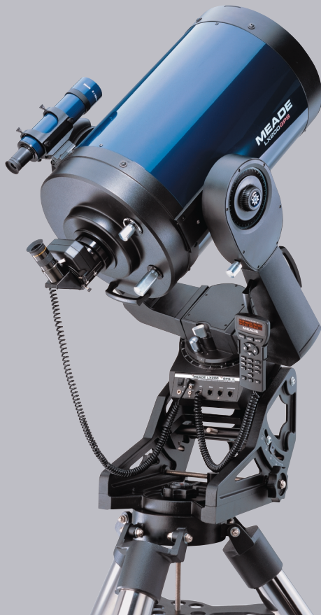
12" LX200GPS, shown on optional Superwedge. The power cord for the standard-equipment Zero Image-Shift Microfocuser plugs into the telescope's control panel.
