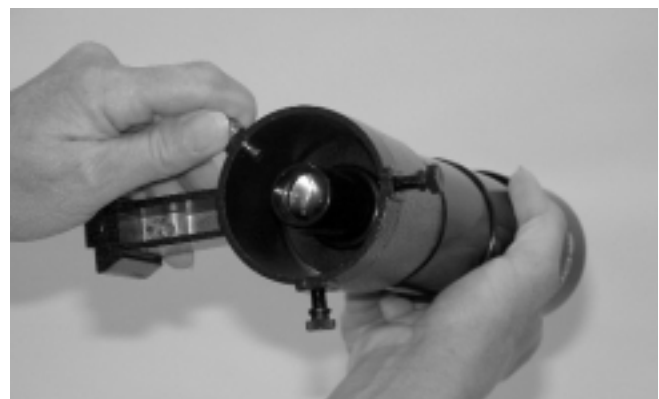
Figure 3b. Pull back on the tensioner and slide the finder scope into its bracket until the O-ring is seated in the bracket ring.
