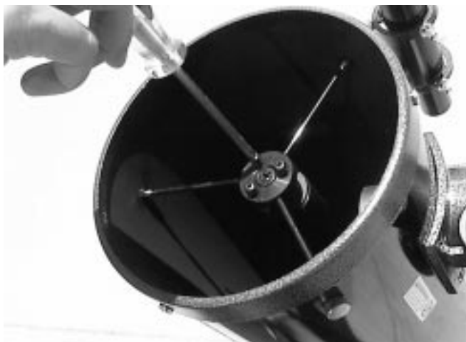
Figure 14. Adjust the tilt of the secondary mirror by loosening or tightening the three alignment screws with a Phillips screwdriver.
