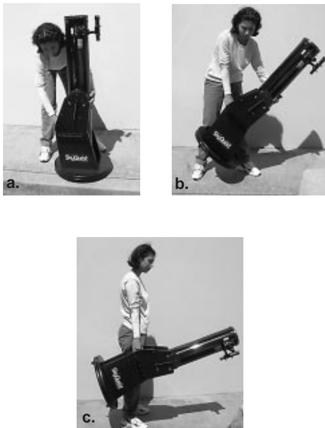
Figure 11. Picking up and carrying the SkyQuest as a single unit (with tube held captive on the base) requires some caution. (a) First, position the tube vertically. Then, grasp the handle on the base with one hand while supporting the tube with the other. (b) With knees bent, slowly lift the base while supporting the tube with one hand. This ensures that the tube will not swing down and impact the ground. (c) As you lift, the whole assembly will tilt down, becoming nearly parallel with the ground, at which time you can let go of the tube with your supporting hand. Make sure you are comfortable with the weight of the whole assembly before attempting to carry it!
