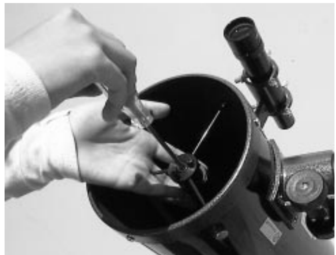
Figure 13. To center the secondary mirror under the focuser, hold the secondary mirror holder in place with one hand while adjusting the center bolt with a Phillips screwdriver. Do not touch the mirror's surface!
