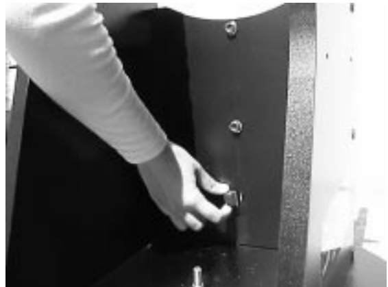
Figure 3. Position the rubber bumper "stop" over the index mark on the inside surface of the front brace.
