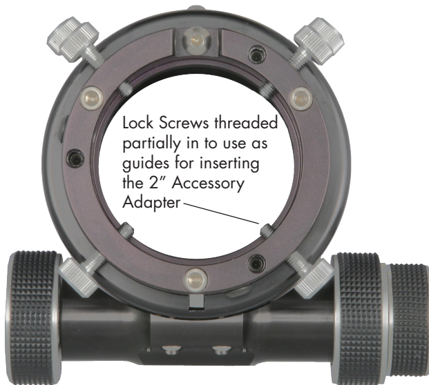
Focuser set to accept 2" Accessory Adapter
