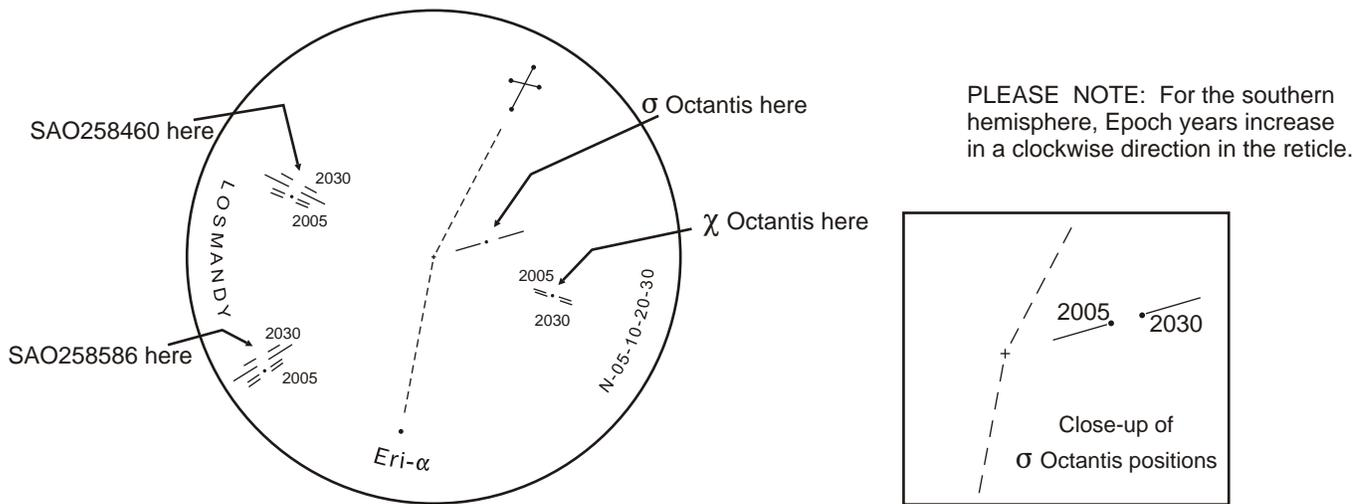
This diagram shows only the reticle lines used for Southern Hemisphere alignment. The 2 sets of lines for  $\chi$  Octantis represent the Epochs 2005 and 2030. The 4 sets of lines for SAO258460 and SAO258586 represent the Epochs 2005, 2010, 2020 and 2030. The gap in the longest line is for 2020, the 2 gaps on the 2 segments counter-clockwise are for 2010 and 2005, and the remaining gap clockwise is for 2030. The stars are diagramed in their Epoch 2010 positions.
