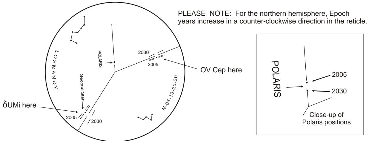
This diagram shows only the reticle lines used for Northern Hemisphere alignment.
