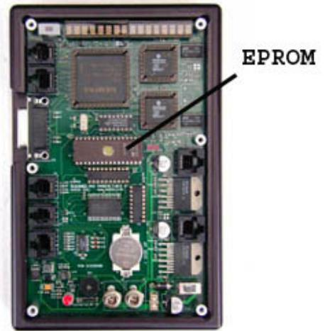
Depending on the contents of the upgrade, you may see the message “CMOS Reset” when you power up the Gemini. This indicates that all parameters have been returned to factory defaults. You will need to follow the procedures outlined in chapter 2 to re-enter all of the setup parameters.
