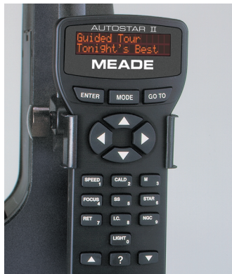
Smart Drive programming is done through the telescope's hand controller.
