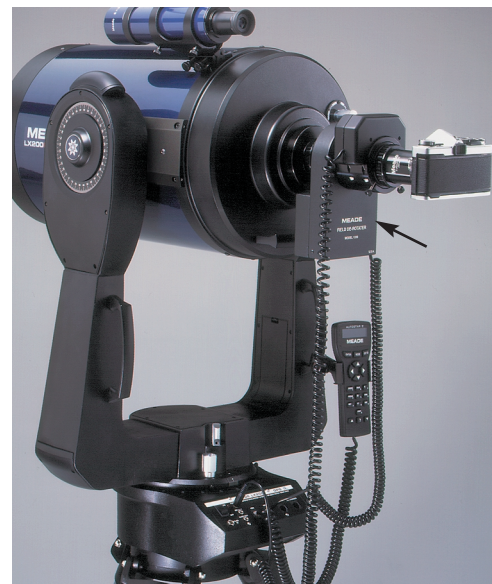
Meade #1220 Field De-rotater (arrow), shown with #62 T-Adapter and 35mm camera body attached to a Meade 10" LX200GPS, ready for long-exposure astrophotography.
