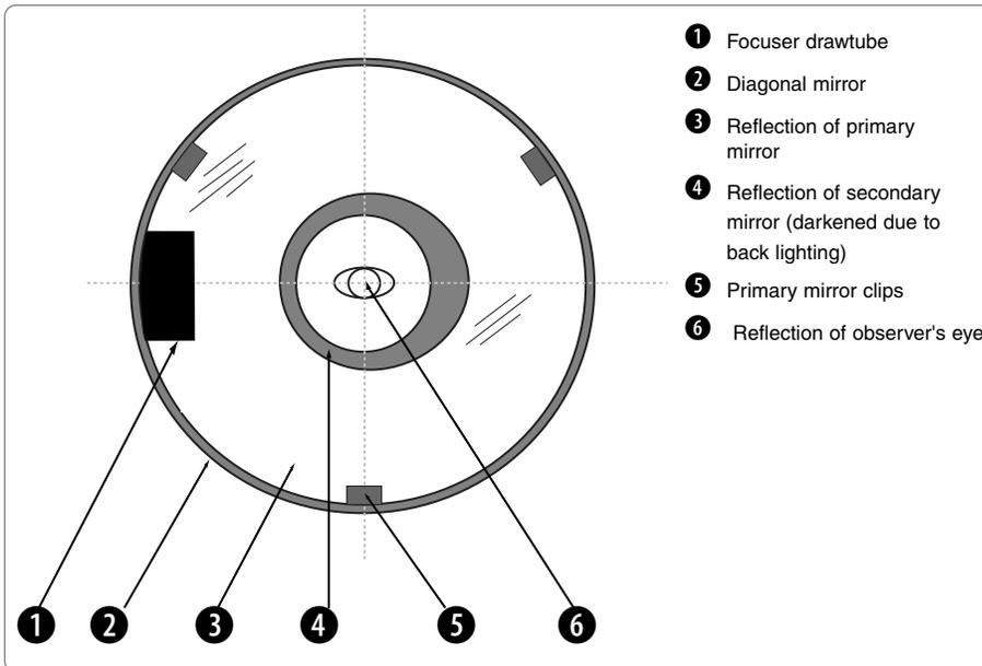
**Fig. D:** The view you will see while collimating a Schmidt-Newtonian telescope.
