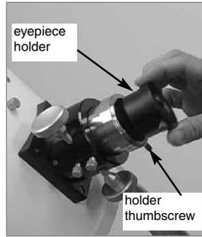
**STEP 11:** Insert the one and one quarter inch eyepiece (1) into the focuser assembly and tighten the focuser thumbscrew (17). To focus the eyepiece, turn the focuser wheels (13) in or out.
