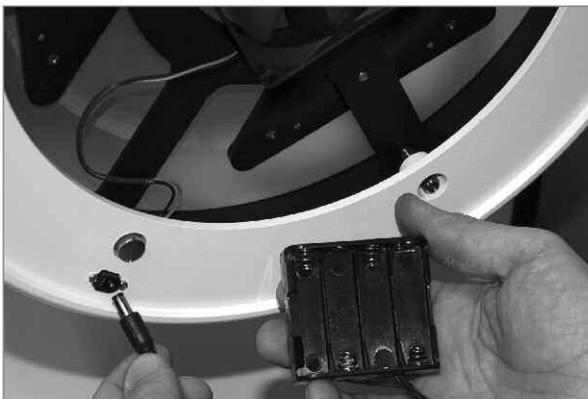
**STEP 14:** Note that there is a fan on the bottom of the mirror tube. It is powered by a battery pack using 4 AA user-supplied batteries.
