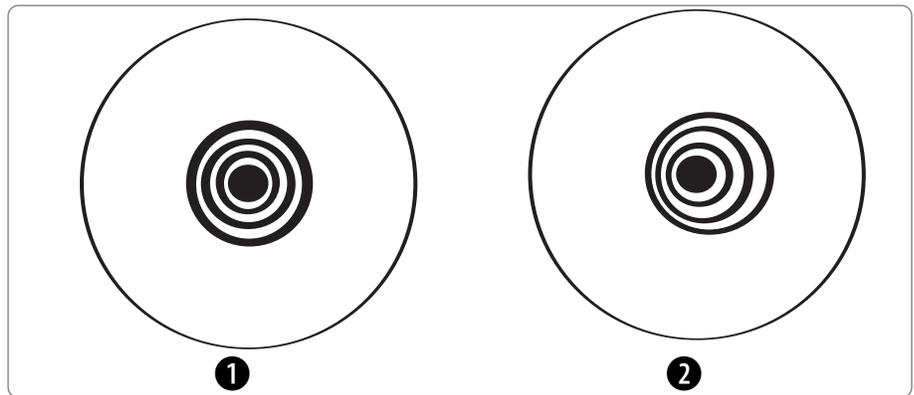
Fig. E: Correct (1) and incorrect (2) collimation as viewed during a star test.
