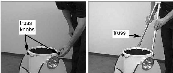
**STEP 8:** Loosen the three bottom truss knobs (6).
