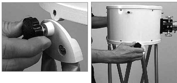
**STEP 9:** After all 3 trusses are in place, loosen the knob (4) on top of each truss.
