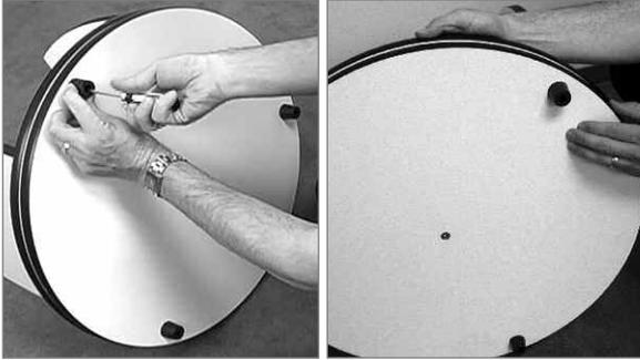
**STEP 5:** Next attach the three feet to the bottom panel. Line up each foot and thread a small attachment screw into the foot to hold it in place. Tighten to a firm feel.
