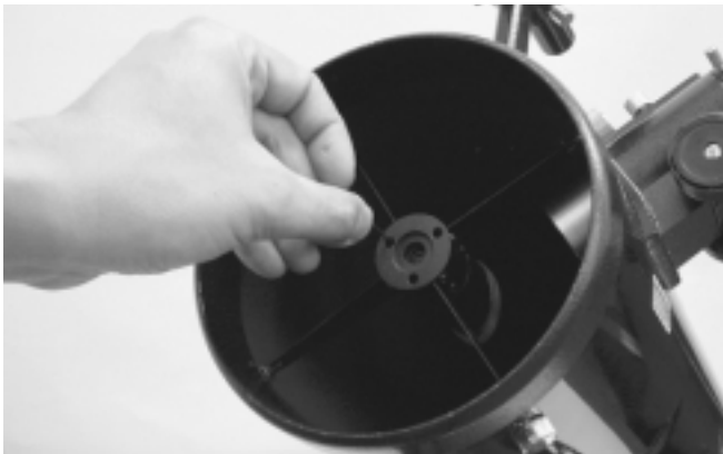
Figure 16. Adjust the tilt of the secondary mirror by loosening or tightening the three alignment set screws with a 2mm hex key.
