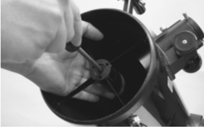
Figure 15. To center the secondary mirror under the focuser, hold the secondary mirror holder in place with one hand while adjusting the center bolt with a Phillips screwdriver. Do not touch the mirror's surface!
