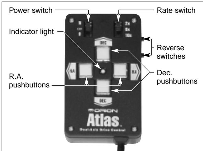
Figure 8. The Atlas EQ Mount hand controller.
