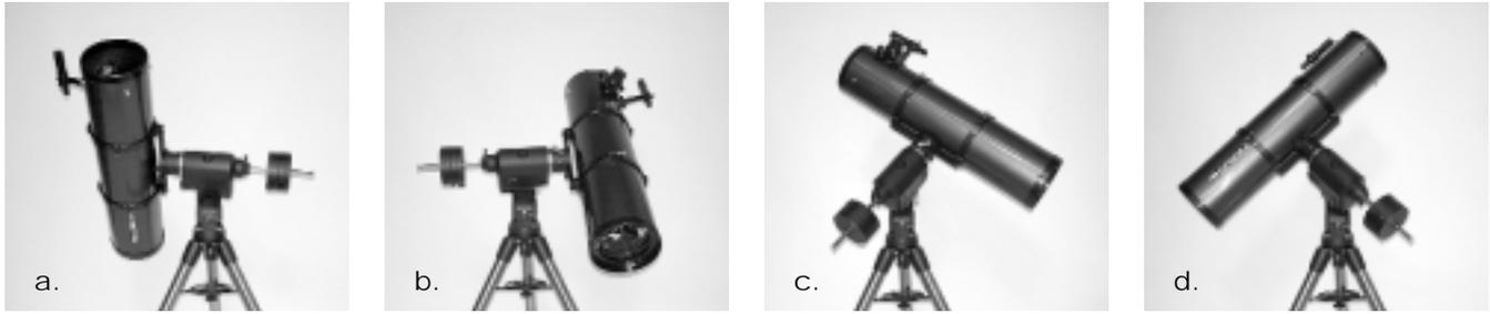
Figure 10a-d. These illustrations show the telescope pointed in the four cardinal directions. (a) north, (b) south, (c) east, (d) west. Note that the tripod and mount have not been moved; only the telescope has been moved on its R.A. and Dec. axes.
