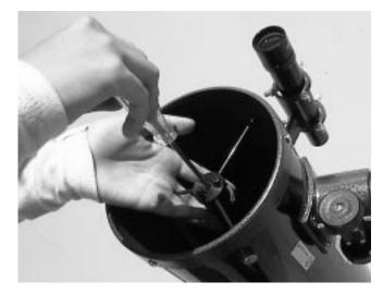
Figure 13. To center the secondary mirror under the focuser, hold the secondary mirror holder in place with one hand while adjusting the center bolt with a Phillips screwdriver. Do not touch the mirror's surface!
