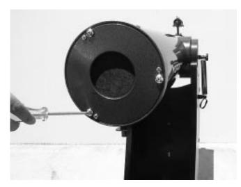
Figure 15. The tilt of the primary mirror is adjusted by loosening and tightening three pairs of collimation screws.
