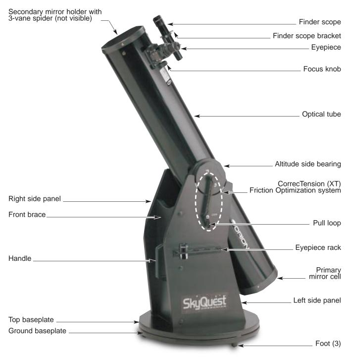
Figure 1. The SkyQuest XT Dobsonian (6" model shown)
