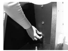
Figure 3. Position the rubber bumper "stop" over the index mark on the inside surface of the front brace.
