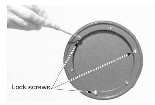
Figure 19. The three screws that lock the primary mirror in place must first be loosened before any adjustments can be made.
