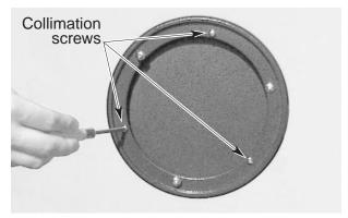
Figure 20. The tilt of the primary mirror is adjusted by turning one or more of the three spring-loaded collimation screws.
