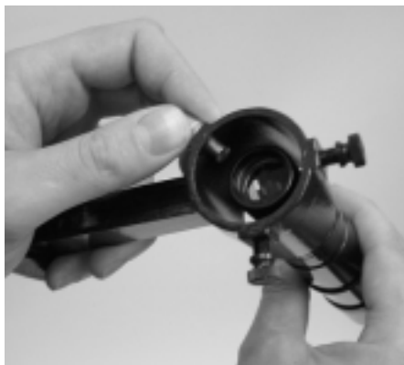
Figure 3b: Pull back on the tensioner and slide the finder scope into its bracket until the O-ring is seated in the bracket ring
