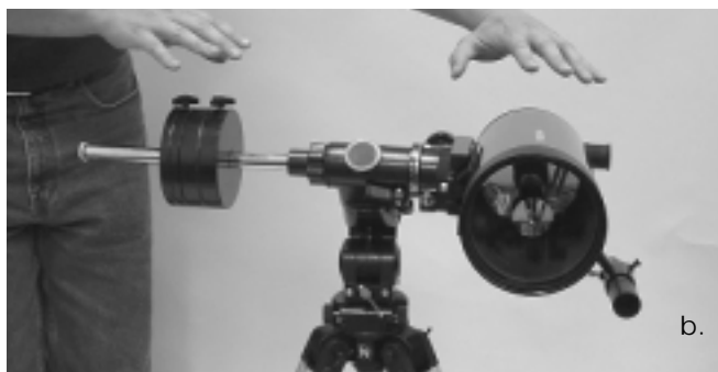
Figure 5a and 5b: Proper operation of the equatorial mount requires balancing the telescope tube on the R.A. axis. (a) With the R.A. lock knob released, slide the counterweight along the counterweight shaft until it just counterbalances the tube. (b) When you let go with both hands, the tube should not drift up or down
