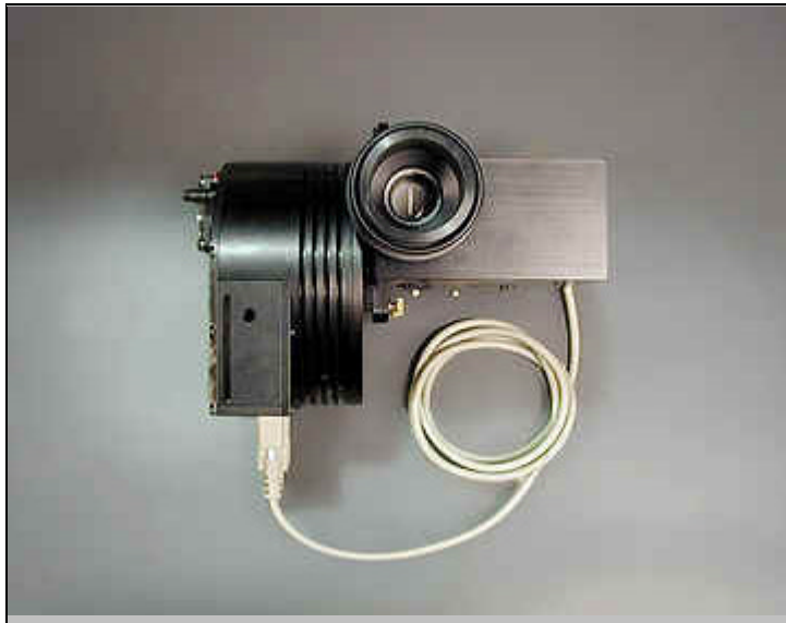
Figure 2. DSS-7 attached to ST-7XME camera
