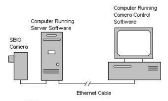
You'll need a computer in the remote site with 32 Bit Windows, an Ethernet card and a Parallel or USB port, depending on the type of camera you have. That's where you run the **ESrvWin** software. On the Local side, you'll need 32 Bit Windows and an Ethernet connection. That's where you run the CCDOPS software. That's all there is to it!
