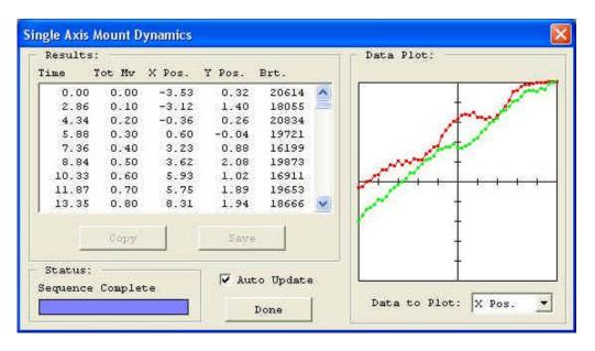
For an absolutely perfect mount with perfect seeing you would see the Green and Red data superimposed upon each other with the plot angling up (or down). A typical mount's results are shown below:
