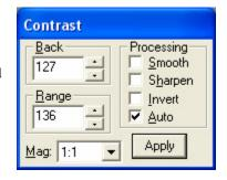
Just for fun click the *Smooth* checkbox in the Contrast dialog. The noise in the image is greatly reduced. The *Smooth* option is handy when for reducing the noise in underexposed images like *Image 3*.
